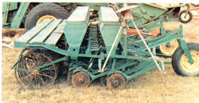
Ryden combined two 12-ft., 7-in.-spaced Deere drills into a single 3 1/2-in.-spaced drill.
